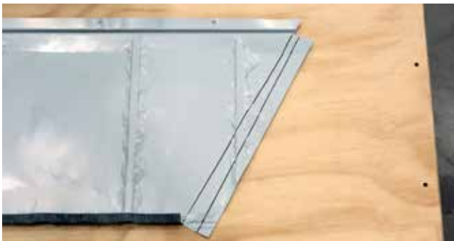
Fig. 21.3 - Panel marked and ready to fold
